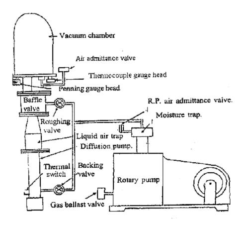
Figure 3.2 Schematic representation of vacuum coating unit
