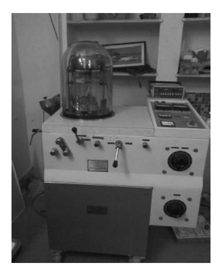
Figure 3.1 Photograph of vacuum coating unit
